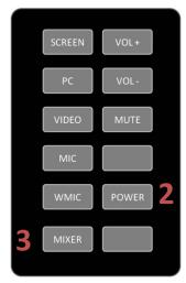
wish to adjust. Next, press the VOL+ button to increase the volume and the VOL- button to decrease the volume.
